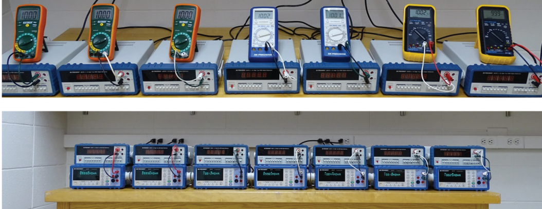
Figure 1. Direct measurement of resistances of DVMs. DVMs may be turned off as long as the buttons are set for voltage measurements.
