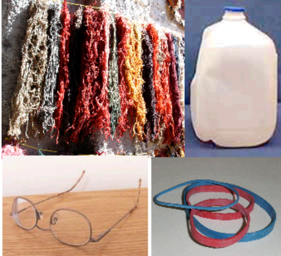
Samples of polymer classes, clockwise from top left: skeins of wool (fiber), polyethylene jug (thermoplastic), rubber bands (elastomer), polycarbonate lenses (thermoset).
